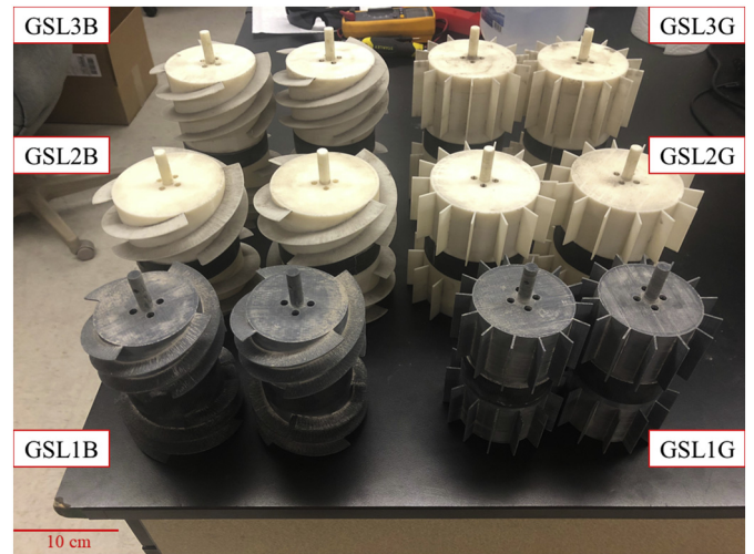
Fig. 2. The wheel sets used in experiments with helical grousers on the left and straight grousers on the right.
