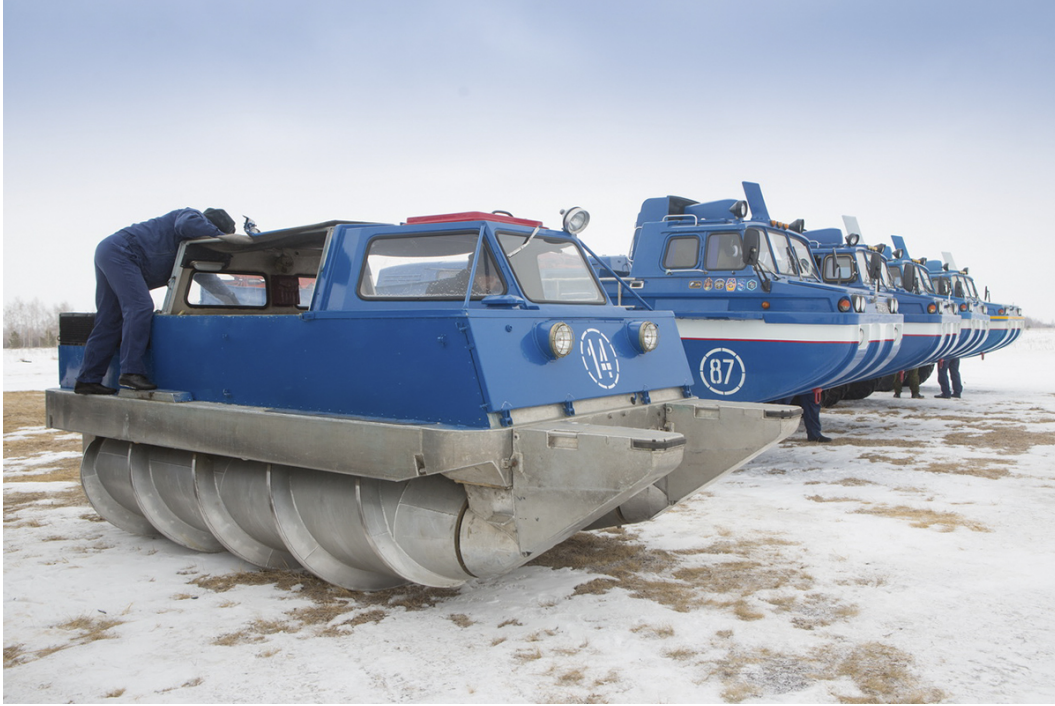
Figure 2. Example of the ZIL-2906 SPV for cosmonaut rescue in Siberia
