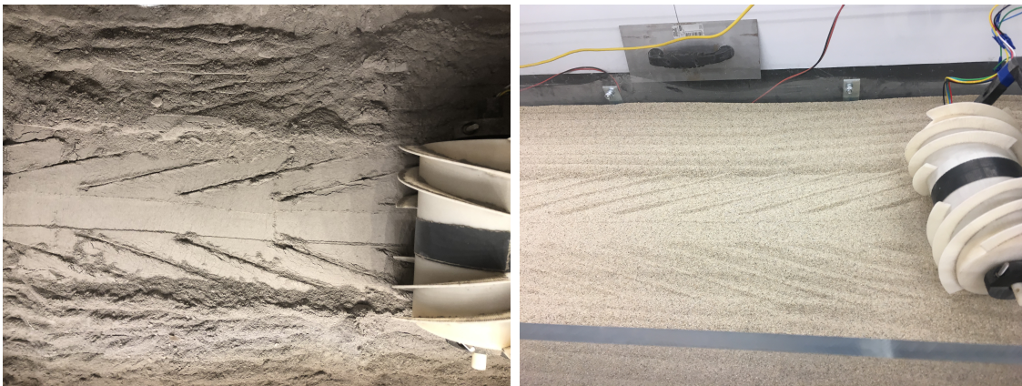
Figure 26. Impression patterns left by helical grousers on both granular media (BP-1 on the left and Quikrete on the right).
