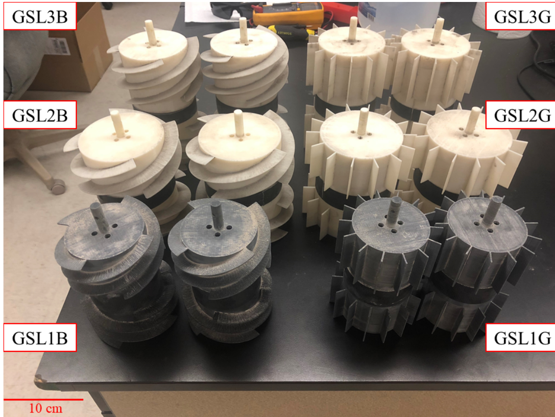
Figure 24. The wheel sets used in experiments with helical grousers on the left and straight grousers on the right.
